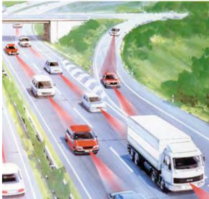
Figure 13.10 ACC Radar sensors for highway and street traffic (Courtesy A.D.C.).
