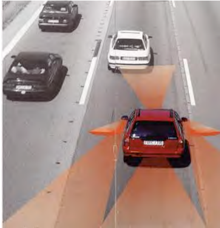
Figure 13.11 Vision of transportation and traffic supported by Radar sensors (Courtesy A.D.C.).
