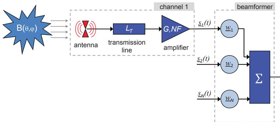
Figure 5.1: Microwave receiver system
