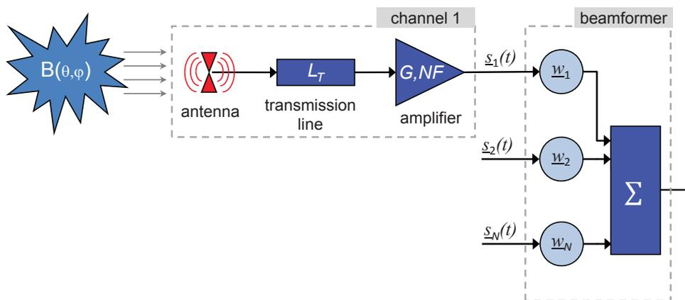
Figure 5.1: Microwave receiver system
