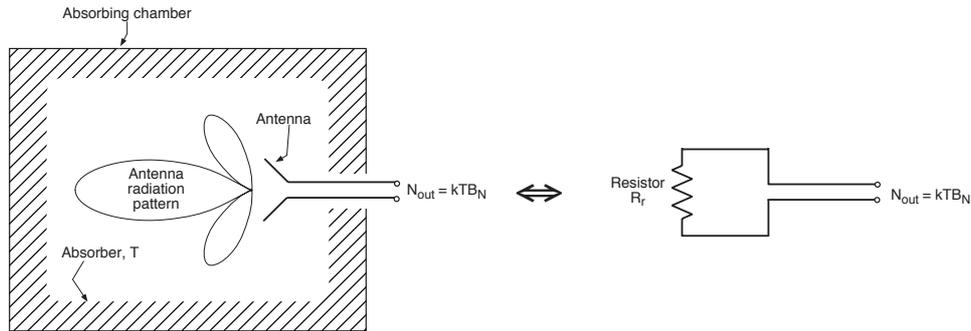
Figure 5.4: Noise power of an antenna placed inside an absorbing chamber
