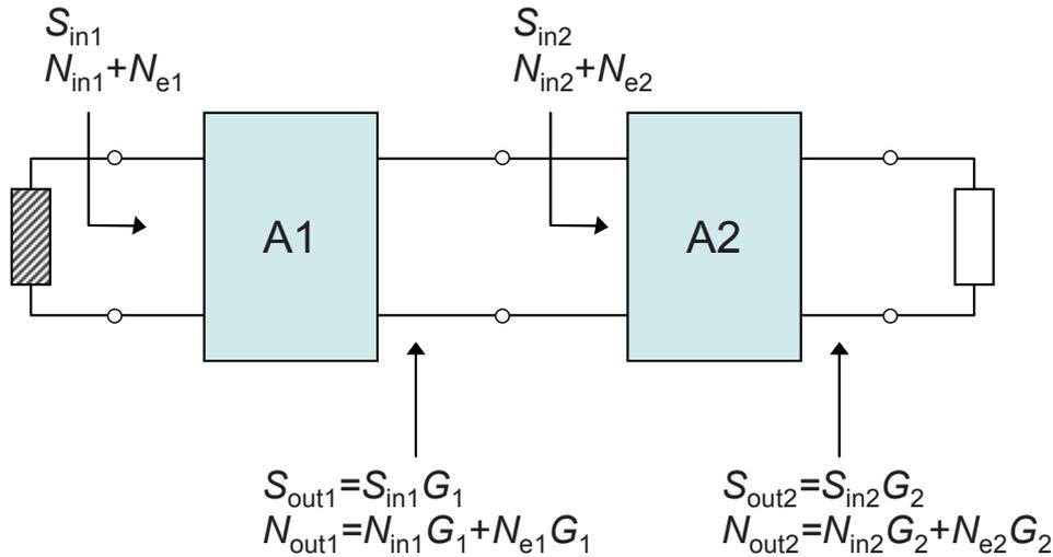
Figure 5.3: Equivalent model for the transmission of noise through a cascaded system
