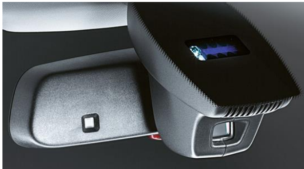
Rain sensor in the rear view mirror
