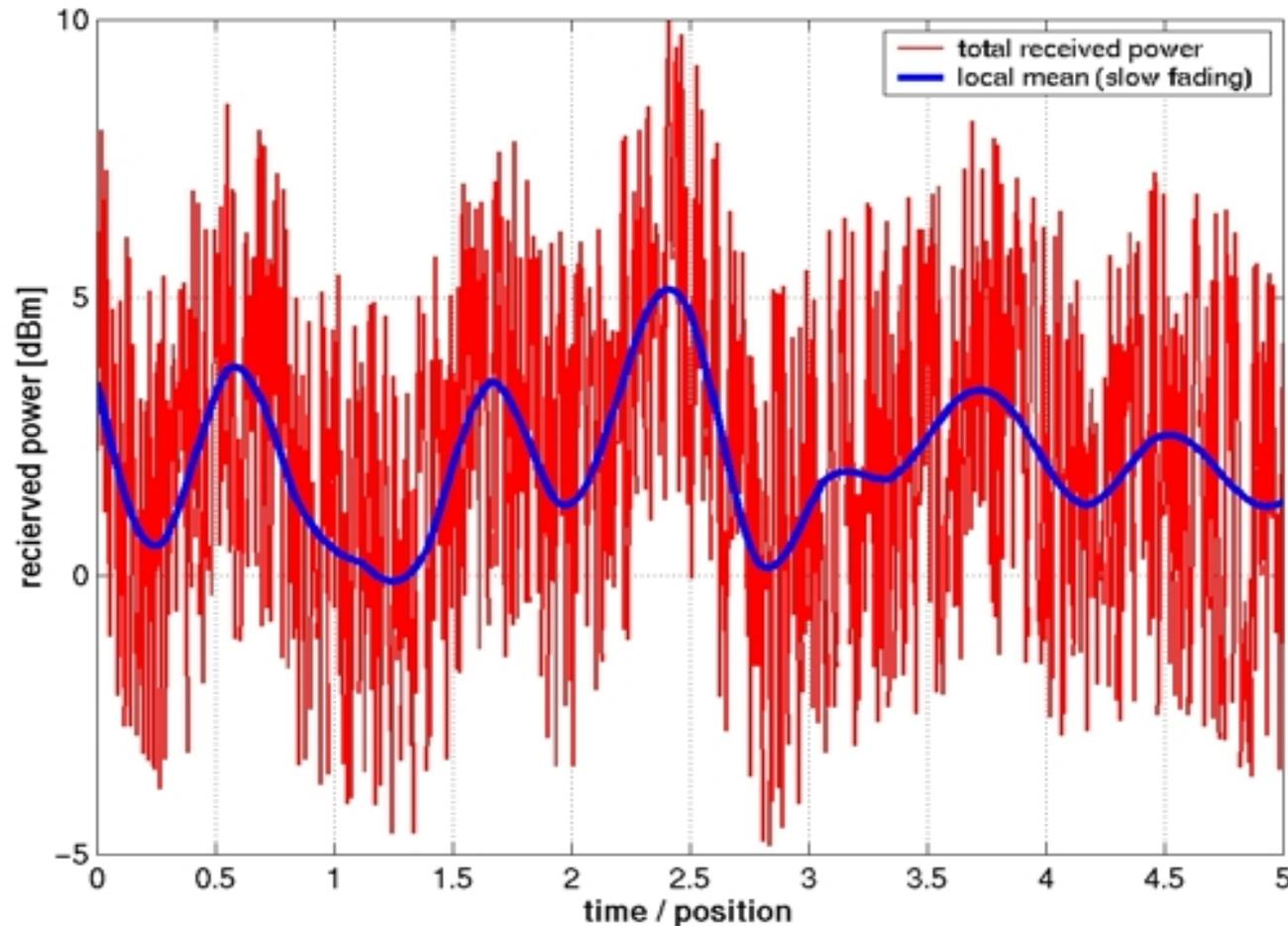
small-scale fading: receiver moving through a spatial interference pattern.
