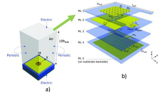
Fig. 5 a) Simulation model of mushroom electromagnetic bandgap (MEBG) unit cell b) Multilayered structure of 6x6 MEBG antenna with SL-to-GCPW feed. See [3] for further details. © Akanksha Bhutani (IHE)
