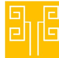
Fig. 4 Electrically small slot antenna. See [4] for further details.
